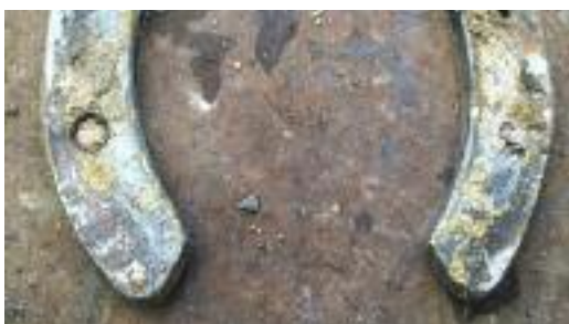
The left hind shoe indicates wear and load is more on the medial side of the shoe. Trim issue?
