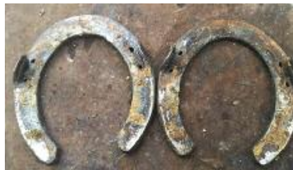
Front shoes showing the wear in the heel area. Even with the lateral modification the heel is sitting to the outside of the web.
