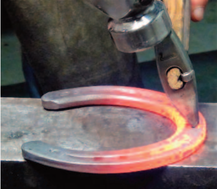
Bloom Wood Handled Bob Punch used to start source material for clip.
