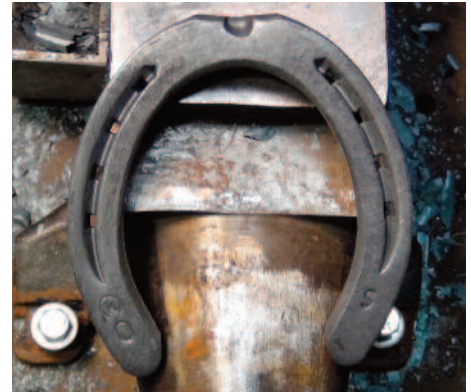
Finished clip from ground surface.
