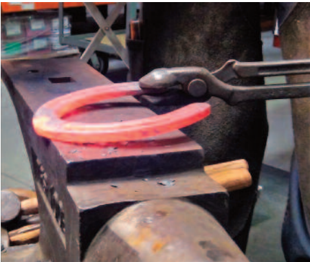
Place shoe over edge of anvil to set base of clip.
