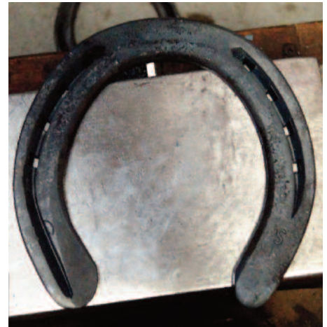
His second step was to forge the inside web of the lateral heel to be sure he had good foot coverage.
