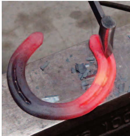
Using a Bloom steel handled creaser, Mike widens the lateral heel.
