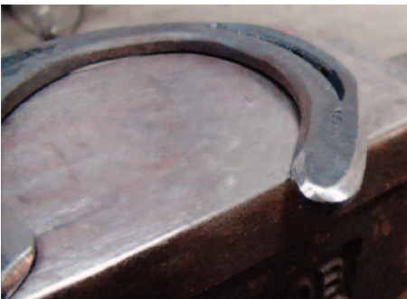
He then narrowed the medial branch on the Baldor to allow it to sink into the ground easier.
