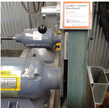
A zirconia belt with material loading present.
