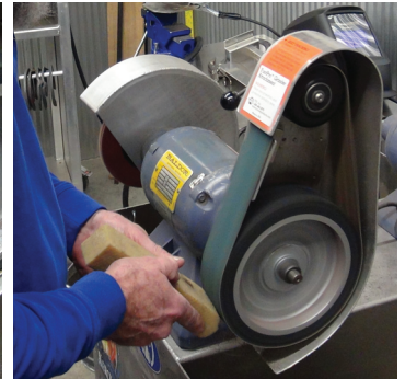
Turn on grinder. Maintain contact with belt and sweep side-to-side to clean.
